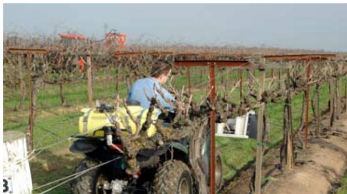
*Using infrared technology, an optical weed control sensor mounted on an ATV emits a pinpoint spray only on weeds, not bare ground, resulting in cost-savings up to 80 percent for weed control.*
