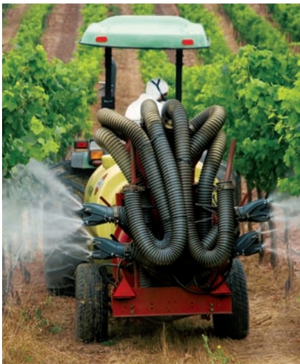
Robert Sinskey Vineyards (Napa, CA) uses a HARDI Arrow B11 pneumatic sprayer to apply Serenade and Sonata and a calcium foliar spray, or wettable sulfur and a potassium foliar fertilizer and a seaweed spray like organic trigger. Drift reduction is achieved as the sprayer-spouts direct the air to where it's needed and nowhere else. The amount of air is adjusted according to the growth stage via a two-speed gearbox. The turbine has a higher capacity than actually needed in most occasions that allows the tractor to run at lower rpm and save fuel.
